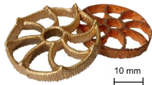
Figure 1: Components made from technically pure copper and a copper-tin bronze using the MJT process.
