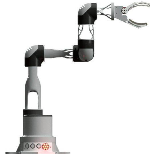
New generation (v1.2.6) LCL robot with circular link cross-sections
