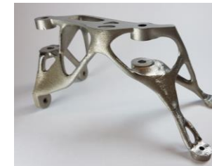
Aero engine bracket with optimized topology. In collaboration with MTU aero engines AG.
